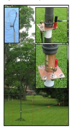
Here's the antenna deployed for action, with close ups of the feed point and the tip. Notice the use of orange driveway markers, both as safety markers and to support the radial wire, and orange streamers to make the radial more visible.
