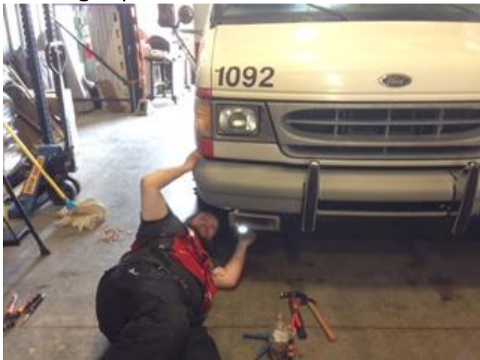
Dan Lott, KF5TQN, replacing a non-functioning PA horn on #1092 ERV.
