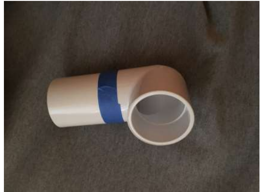
Elbow and Extension Resonates About 600 Hz
