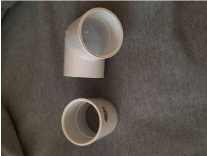
Elbow Alone Resonates About 850 Hz
